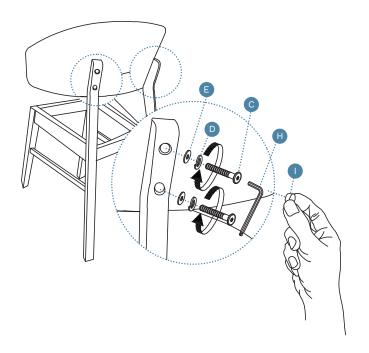
Attach 1 x backrest to assembled frame and secure with 4 x screws (C),  $4 \times 1$  x spring washers (D),  $4 \times 1$  x washers (E). Tighten with an Allen Key (H). Once tightened insert  $4 \times 1$  wood buttons (I) as shown.
