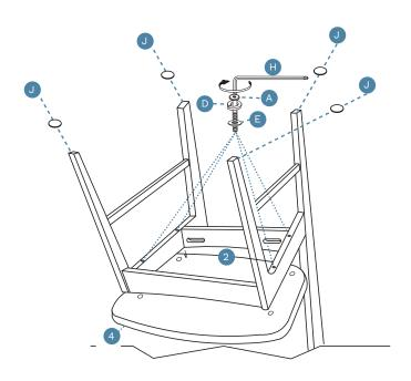
Attach seat (4) and frame (2) together as shown and secure with 4 x bolts (A), 4 x spring washers (D) and 4 x washers (E). Tighten with an Allen Key (H). Once tightened attach 4 x felt pads (J) as shown.
